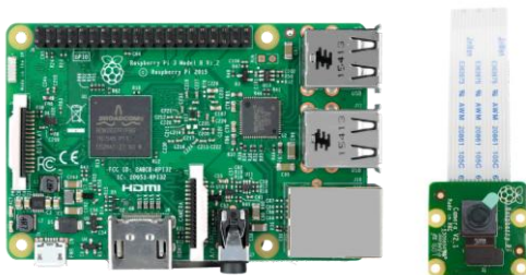
Figure 2: Raspberry Pi 3 Model B and Camera Module [9]
