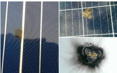
Figure 1. Hotspot's effect on Solar Panel [14]
