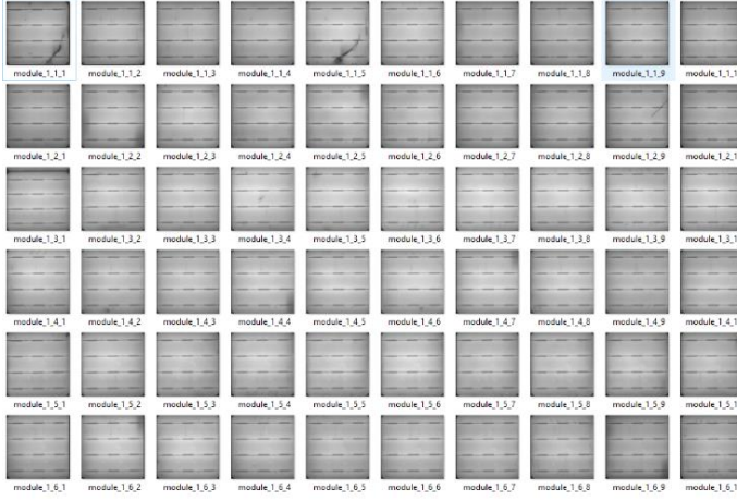
Figure 6. Cell-based fragmented images of a 60-cell solar panel
