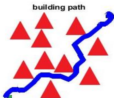
Fig. 4. Building The Final Path That Make The Robot Reach The Goal State.
